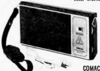
"COMACHO" EIGHT-TRANSISTOR RADIO. Kit provides basics of superheterodyne transistor theory operation. Builds into an attractive printed circuit-board radio, mounted in plastic case. Compares favorably with more axpensive units. Earphone included. \$19.95 each.
