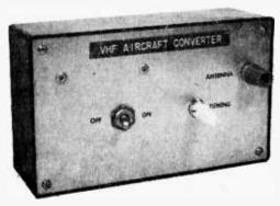
To receive aircraft signals, simply place your BC radio near convertor and move it about slowly until the radio peaks at its maximum volume. Tuning it will be a slow process.
