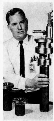
Used for seismic measurements, digital-air gun by Texas Instruments (above) is electromechanical device that forces air bubbles of predetermined sizes under water. Below, shipboard oceanographic system, also developed by Texas Instruments, digitizes, corrects, linearizes, arranges, and plots variety of data.
